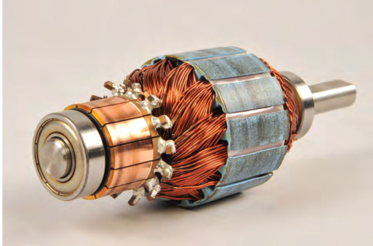
Figure 22. In real dc motors, the armature (rotor) is made up of several wire loops and the commutator has several segments.
